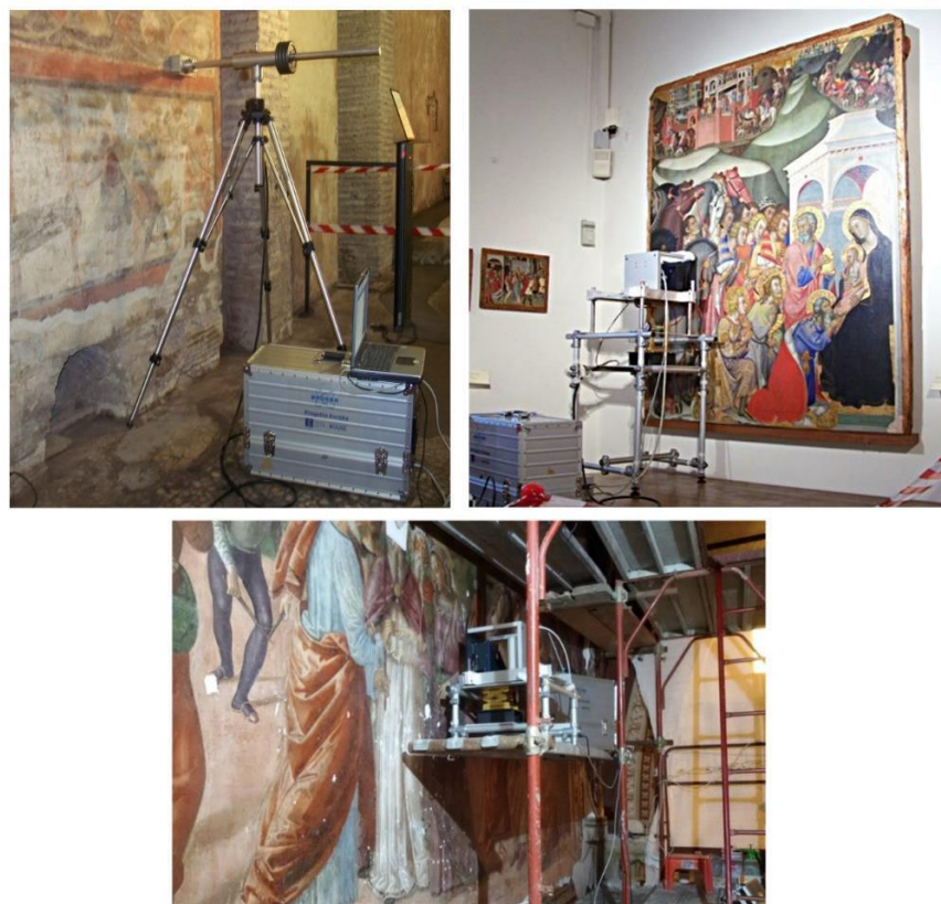
Figure: NMR probe mounted on its metal arm and support while measuring paintings.
