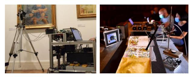
2. ASD FieldSpec® 4 Hi-Res High Resolution spectroradiometer (350-2500nm), Malvern Panalytical
