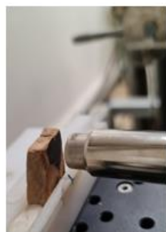
Fig. 1 GI-XRF: Attic ceramics. By recording the XRF signal in an angular scan of the shown fragment, the chemical composition of the black surface gloss (rich in iron, titan and potassium) is separated from that of the red ceramic core (rich in calcium).
