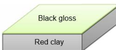
Fig. 1 GI-XRF: Attic ceramics. By recording the XRF signal in an angular scan of the shown fragment, the chemical composition of the black surface gloss (rich in iron, titan and potassium) is separated from that of the red ceramic core (rich in calcium).
