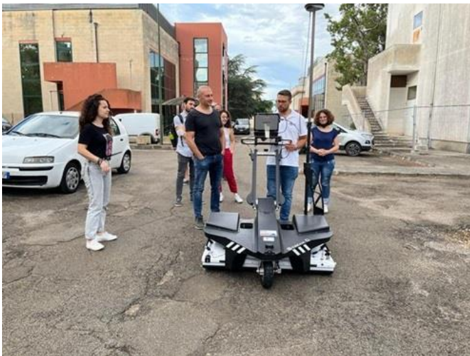
Figure: georadar stream C
