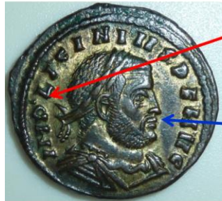
Detection of the 2 \mu m thick Ag-Hg surface enrichment patina in a Roman coin composed of Cu-Ag.
