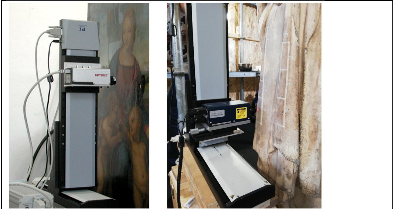
Figure: Microprofilometer during the in situ measurement of painting (left) and of a statue (right).
