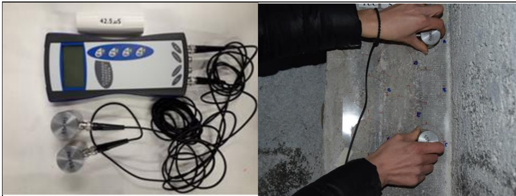
Figure 2. (left) Matest C369N ultrasonic instrument; (right) in situ test at the War Memorial Tower (Torricella Peligna, CH)
