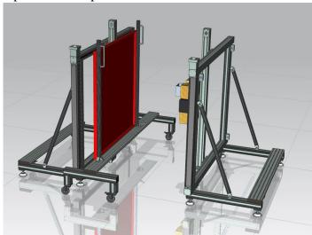
Figure 1: On the left, the unit for the detector handling; on the right the one for the X-ray tube.
